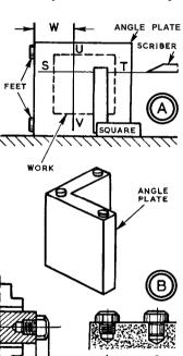
To check the depths to which feet must be machined, set the angle plate with its faces vertical, using three pieces of material like silver steel rod, with shimstock packing. In facing feet, which is the last operation on them, they are screwed one at a time in a holder. A zero setting is taken from the face of this for the top slide collar; and the tool is set at X for the shallowest foot, and to X plus n thou for the other two. The material can be
