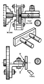
at C has the advantage that it extends below the centre line of the lathe spindle. Construction is very simple, with proportions to suit the lathe: two pieces of steel rod are screwed firmly into a flat plate.
