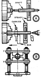
of similar material attached to locate in the bed. Two substantial studs are fitted to the top side (shouldered into holes, riveted and brazed) to take locknuts for setting the steady jaws or bearing. For general work, the bars, T and
