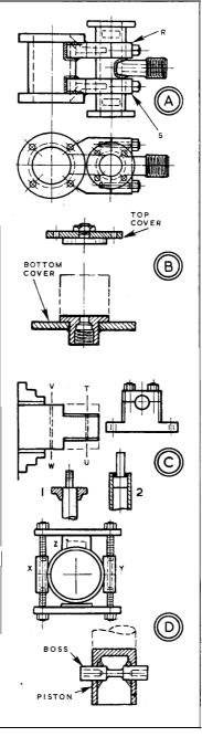
the piston valve cylinder is mounted in them by clamps. With this construction, the blocks can be prepared. They can be bored and radiused, the ports can be cut in them by drilling and filing or milling, and matching ports can likewise be made at the ends of the cylinder.
