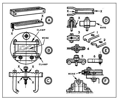
material can be used for clamping, if a stirrup is made for each bolt D. Bars can then be cut to length for each job. To make a stirrup, flat material is turned U-shaped by hammering it over a block equal in thickness to the combined dimensions of the bars and bolt. After this, it is squared to length by filing, and brazed or welded to a plate X. Holes for the bolt should be easy, and the hole in the plate may be larger still, to allow for lengthwise tipping in adjusting and clamping.
