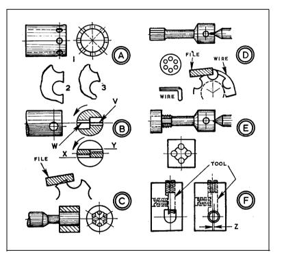
the material centre, and this is done when drilling the opposite side. Finishing to the centre can be done with a flat-ended drill; then when the material is faced, as at B, the tips of the teeth are left radial, V and W, to provide free-cutting right to the centre-with the shaded areas relieved by filing. An endmill made by filing two flats on material has tips of teeth on planes X and Y.
