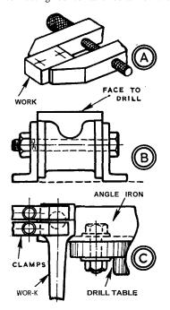
cap, as at C. Such work can hang down the side of the drill table, where there would probably not be sufficient space for it to stand on top. Two clamps may be needed for a connecting-rod and cap, as shown. The angle iron is bolted to the drill table with this slewed round, to align each centre punch dot in turn beneath the drill point.
