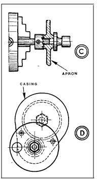
tempered and fitted to its mandrel. Having dismantled the saddle, or at least removed the apron and sawn off the surplus length of the boss, the remainder can be faced back flush, as at C, backing up the apron by a pad centre, and applying feed from the tailstock.
