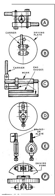
of a definite size, a clamp type carrier can be made to grip full circle, as at B, by drilling out to the diameter-or reaming if required. To give grip, drilling and reaming can be done with a piece of paper between the faces of the carrier, or one face can be eased afterwards with a file.
