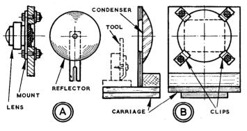
However, distributing the light evenly over an area to cover the plate or film overcomes this defect; and in the same way a profile anywhere in the lighted area, such as that of a contour gauge, can be clearly seen. It is done by using a condenser next to the light source, the bulb; then whatever is to be projected-a film or a tool-is placed for focusing between the condenser and the camera or the projection lens.
