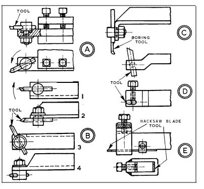
A holder of angle-section material to use in a turret and admit of setting tool edges to centre height, can be as at B, 1 and 2. The flat side of the holder stands vertically with nothing lower than the clamping face of the furrat to obstruct rotation. Tool clamping is similar to that of the other holder.
