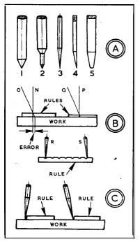
1/8in. or 5/32 in. silver steel rod, the point must be long and fine, as at A (3). To avoid breakage, it should be used at moderate, pressure; and where conditions demand considerable force for scribing, a blade-type tool, as at (4) and (5), is preferable. It can be from flat-stock, chamfered one side, tapered, and with a small radius at the edge.
