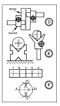
Centres of round stock may be found with the centre head or a square, as at E (right), or in V-blocks (left), using a surface gauge. With the centre head, intersecting lines locate the centre, but with V-blocks, it can be "boxed" if required.
