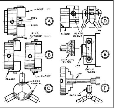
to fit clamps, as at B. For securing jaws inside the chuck diameter (right), each clamp can be straight and balanced by a small packing block. For securing, however, where jaws stand proud of the chuck diameter, each must be bent down (left). In both cases regulation of individual holding screws is necessary.
