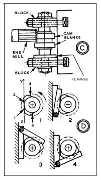
after milling the first flat, a gauge (set to angle from a protractor) can be presented to it and to the edge of the mounting plate, to locate the blank for the second flat. Finally, to finish the base circle, the cam can be held between two thick washers for filing.
