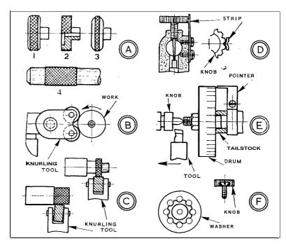
the head giving support each side. A narrow knob or handle is easiest on which to produce a good knurl, as the wheels can be run straight on, as at C, right. Any slackness on a wheel, allowing it to tilt, left, is almost certain to cause trouble on a long knurl.
