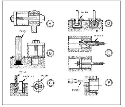
the most suitable materials to mate with shafts or pins in particular locations-whatever materials may be used for constructional parts. Thus, bushes may be of white metal, brass, phosphor-bronze, gunmetal, or hardened steel.
