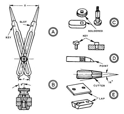
to 1 in. 1 ft. For working on the photograph, X would be kept at driving wheel scale size on the steel rule, while dimension Y is adjusted to the diameter. on the photograph. Other dimensions will thus appear at 1 in. 1 ft. Briefly, one can adjust the proportions as necessary for this or any other scale.
