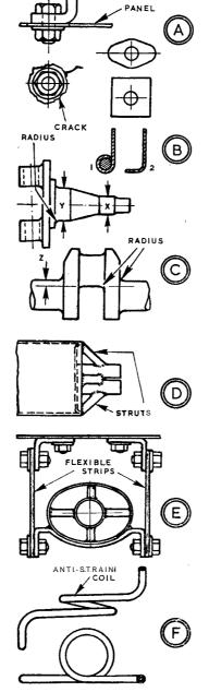
strain and vibration can be verv prone to cracking; and unless there is some support for a panel at a bracket, a crack may completely encircle a bolt, as at *A*. In these circumstances large washers can effectively distribute strain over a wide area. They may be round, oval or square.
