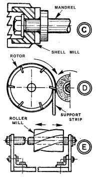
the saddle below the wheel, as at D Each tooth or blade, is then kept down to the support as the saddle is traversed.
