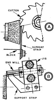
on the vertical slide when a lathe is used. Such a jig may be made by boring a hole for the mill shank in a block of material like aluminium, and fixing a support strip by screws. A collar each side of the block locates the mill, while permitting rotation from tooth to tooth. For a larger shell mill, as at C, a mandrel must be provided to mount in the jig, though the principle is the same.
