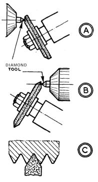
with the shaped grinding wheel substituted for the screwcutting tool and fed into the work from the cross feed, and the saddle traversed by the leadscrew. Using a jig, the grinding wheel is run in the chuck, and the work is mounted and rotated in a holder.
