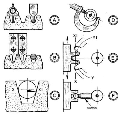
A check on depth of tooth or thread is possible using any simple depth gauge, as at A, left, first removing any burrs with a smooth file Depth setting for such a gauge can be from a disc or ring faced in the lathe, tied, or lapped so it can be laid on the surface plate with the depth gauge on top.
