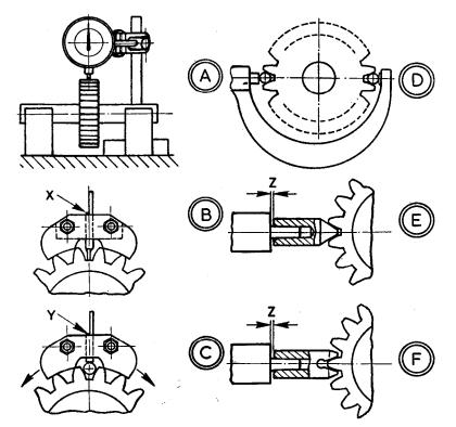
of the gear, would indicate an over all eccentricrty, with the teeth cut, or generated about another axis.
