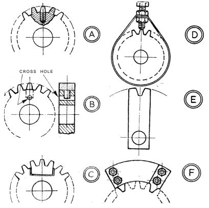
tapped for a piece of studding to be screwed in which can be filed to tooth profile. On a broad gear, two or more pieces can be fitted in this way; but whatever the width of the gear, there is always a loss of tooth width from the metal which must be left outside the stud holes.
