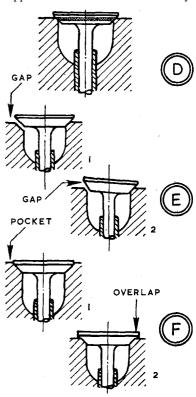
seating El the valve nevertheless shows a continuous seating. A good seating E2 is marked all round by a faulty valve, while a faulty seating and faulty valve may be misleadingly well marked.
