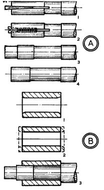
set up can be lapped holding the lap by hand, especially where such part may be a bush difficult to hold otherwise. The lap may then be somewhat shorter than when it is itself run in the lathe and the part applied to it.
