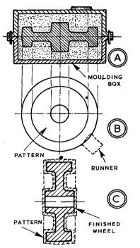
not necessarily machined all over an allowance must be made for metal shrinkage. Per foot of length, this allowance is 1/10 in. to 1/8 in. for cast iron; 1/8 in. to 3/16in. for aluminium and 1/5 in. to 1/4in. for brass. If desir al "contractio n" rules can be used on which all dimensions are these proportions overlength.
