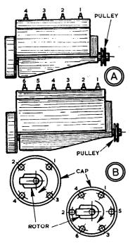
corners like a square nut-while the cam of a six-cylinder engine has six lifts or corners, like a hexagon nut. On each lift of the cam operating
