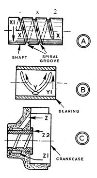
In the same way oil can be displaced between a shaft and bearing, or between a boss and the bore of an enclosing casing.
