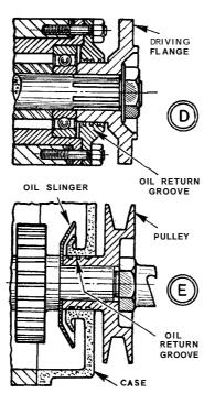
Thus, on the most elementary view, if it is a case of lubricating the shaft and bearing, the point of entry of oil should be to the right, so it is carried into the bearing; if the point of entry is on the left, oil will continually be drawn from the right side, which may not receive enough. On the other hand, such a thread would prevent loss of oil towards the right from a casing on the left. To maintain these effects
