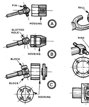
the housing usually has both ends open, and is bolted to a flange on the driving or driven shaft—otherwise, with one end closed, considerable difficulty would be experienced in producing true parallel-sided slots.
