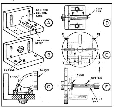
An ordinary sideways setting is obtained by marking a vertical line up the component face from the base. Then with the component clamped, the angle-plate is turned into a vertical attitude, and the scriber point of a surface gauge is set to the line. Tuming the faceplate through 180 deg and testing again, the line should coincide with the scriber point when the setting is accurate.
