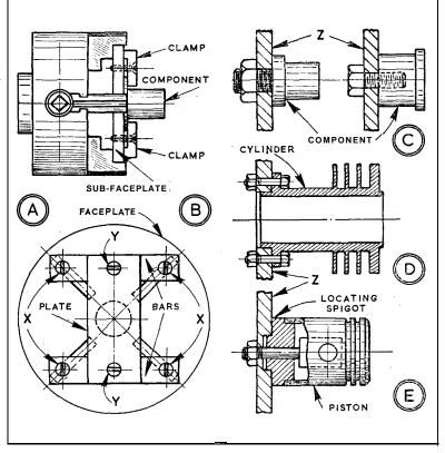
for sub-faceplates in the form of parallel discs for holding in the fourjaw independent chuck, or flat rectangular bars-for similarly mounting -or attaching to the normal faceplate. Aluminium alloy, brass. and mild steel can be used; and the most convenient thicknesses are 1/4in. to 3/8 in. If desired, a simple casting could be obtained from a wood pattern and machined.
