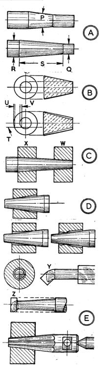
when the work is mounted between centres. Again, on lathes so equipped, a taper turning attachment may be used to control movement of the cross-slide, leaving the work in longitudinal alignment with the lathe bed.
