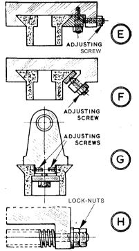
stock lateral adjustment as at G. The tongue portion of the headstock fits with slight clearance between the guide faces, and has two adjusting screws each end which can be turned outwards to wedge between the faces. Thus, by regulating the screws, the headstock can be trued laterally to produce true turning or boring in the chuck.
