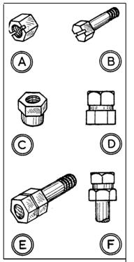
A deep bolt head, like a deep nut is often all that is required to facilitate assembly and dismantling. Special bolts can be turned from hexagon bar, a somewhat lengthy and deterring process, and another method, quicker and generally equally effective, is to braze an ordinary nut on top, **E**. If the double-hexagon principle is required a nut as C can be used on the bolt somewhat shortened, **F**.
