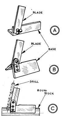
If required, a machine without a built-in level can be aligned in this manner, placing the level on the drill before commencing, then re-checking when the hole has progressed a little way but not so far as to prevent correction if necessary. Yet another method is to hold a small square to the work and align the drill to the blade.
