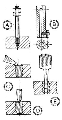
IN ASSEMBLIES where bolts would be impracticable, study are an alternative to setscrews and, being permanently fitted, possess advantages.
