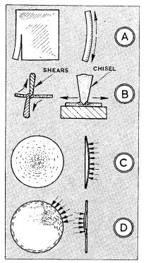
"oil can bottom," when if the perimeter is held the centre can be pushed one way and the other. Hammering the edge, however, particularly if not all round, renders this unstable, **D**, and laying the disc on a flat surface shows the edge to be upstanding in places. Pushing these down causes spring-up in other places
