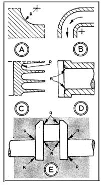
sistance than a continuous straight flow; whereas if the bend is a sharp comer, the edges set up minor contrary flows or eddies.
