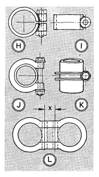
internal diameter required or bored out in a lathe to size. The boss for bolt or screw can be smaller tube or rod drilled out, the hole being continually cleared or tapped halfway for a setscrew. Filed on the outside to suit the diameter of tube or washer the boss is then brazed or welded on. Finally, boss and tube are cut through. Diagrams H and I show end and plan views of a clip made from steel tube. One from a washer would be narrower, with the boss overlapping the sides.
