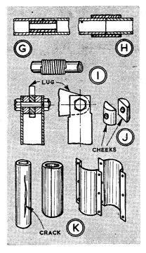
because of the easier and more uniform heating-that is, a solid plug may not heat sufficiently for the brazing to run through the joint. A pipe which is cracked may be repaired and strengthened by binding with clean wire, then soldering over, I.
