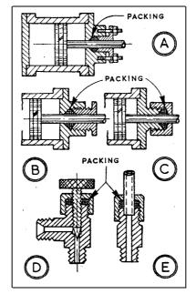
taps), and small needle valves, **D**. In the latter connection, it can be said that the packing will compress and seal in the thread, as shown, providing it is true and smooth, and an important saving in length can be made, by comparison with valves having a plain diameter for the packing to bear on.
