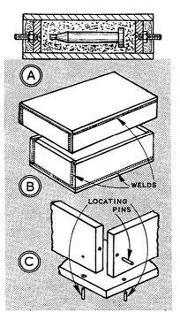
washers, and components on which distortion may be small or not important, can be case-hardened singly or in numbers by laying on a piece. of sheet iron, heating to red, covering with compound, reheatmg, then quenching the lot. A shaft or spindle, however, on which distortion can occur, should be lifted off by pliers, plunged vertically and kept moving.
