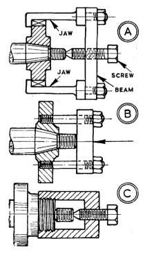
sprockets and consists simply of three suitable bolts and a bar. The latter is drilled clearance, centrally for the pressure bolt, and at suitable spacing for the bolts acting as jaws to lie holding firmly in the sprocket teeth.
