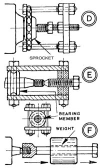
hole for a screw as shown. This puller is intended for drawing inner members of ball bearings, and holes are drilled in the top and bottom plates for the two bolts passing through to hug tightly in the semicircular track of the race member. Two bolts also attach the endplate for the pressure screw or bolt. The type at **F**, known as an impact
