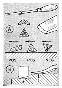
The triangular scraper is similar, but the blade is three-cornered, running to a point. Though the blade tapers, the edges are not straight, but slightly curved, so a surface can be touched by a portion of the blade-though less easily than with a bearing scraper. This scraper is often in small sizes with a knurled handle.
