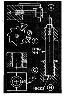
In all reaming, maching or hand, rotation is very slow and ample power is essential. In hand work, either the component is held in the vice and the reamer turned with a substantial tap wrench, or the reamer' is held and the component turned-when it is a size and shape permitting proper leverage.
