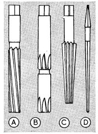
is for opening out drilled holes to take taper pins-as when a collar is pinned to a shaft, the pin then driving in firmly. A machine reamer E has short normal cutting blades, an axial slit and a coned central screw for adjusting with a pinspanner to regulate the size.
