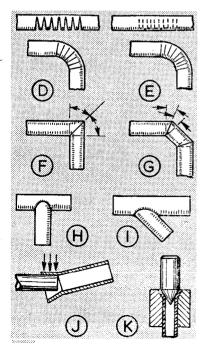
Copper and brass pipes of small diameter butrelatively thick-walledcan be bent easily unless the radius of the bend is very small. For a bend of minimum radius, the material should be annealed, i.e., heated to red and quenched in water. steel pipes should be bent at red heat unless the curve is very gradual, when cold bending is possible.
