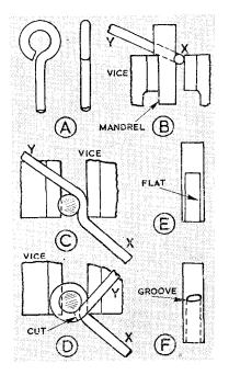
bent at right angles. Hard brass and copper, common iron and duralumin are most prone to cracking when working. The first and second should be annealed, the third worked at bright red heat and the last avoided except, for large-radii bends-or when heat treatment is possible.
