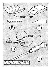
producing a flat for clearance at each cutting edge. On a very tiny drill the flats can be produced rubbing on an oil'stone, or hand-honing with the drill in parallel-jaw pliers.
