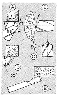
Thin oil, such as cycle oil, should be used on an oil stone to float particles of metal away;, hand hones may also be fed with thm oil and both types, when dirty and clogged, can be scrubbed in paraffin. As with grinding wheels, the area of working should not be restricted for the hone or stone to become locally worn.
