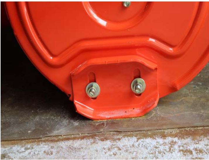
Figure 2 – Ariens Snowblower with Factory Skid Plates
