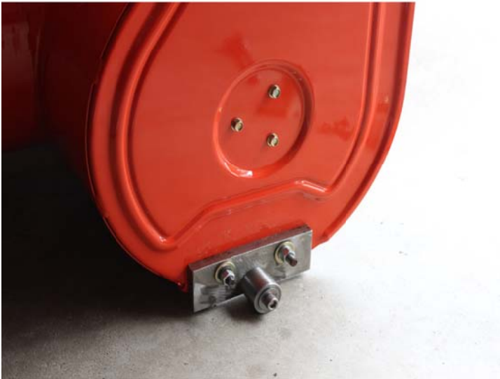
Figure 3 – Ariens Snowblower with Custom Stainless Rollers
