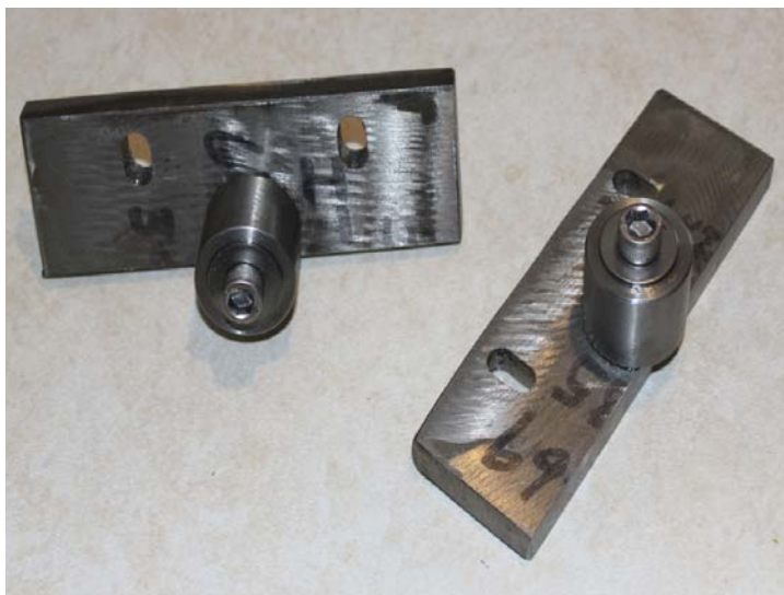
Figure 1 – Completed Stainless Rollers, Ready For Installation
