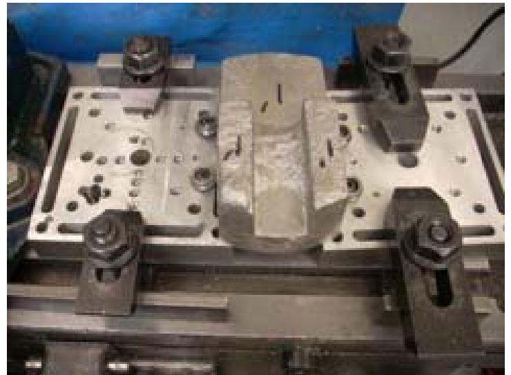
Holding Casting Photo by R. G. Sparber
