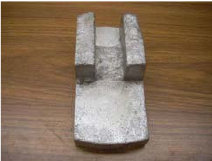
Removed Gate Photo by R. G. Sparber
