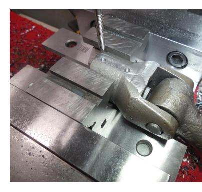
Second side was easier. By a fortunate quirk of inanimate objects, the slightly protruding pivot pin of the vise handle lined right up with the vise (being used) jaw screws, and the little bit of recess there. So I didn't need to pad the part itself to get past that protrusion. It's sitting on a 1/4" thick plate underneath so the two sides end up essentially parallel. But really, nothing here is terribly critical.
