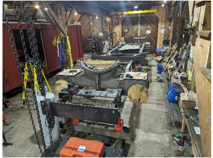
This is the frame of what will be an operating 2 foot gauge operating live steam locomotive
